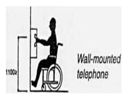
Fig-3. Telephone Stand & Wall Mounted Telephone
