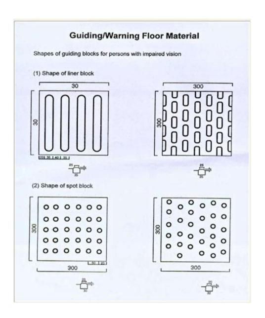
Fig-2. Details of Guiding/Warning Floor Material for persons with impaired vision.
