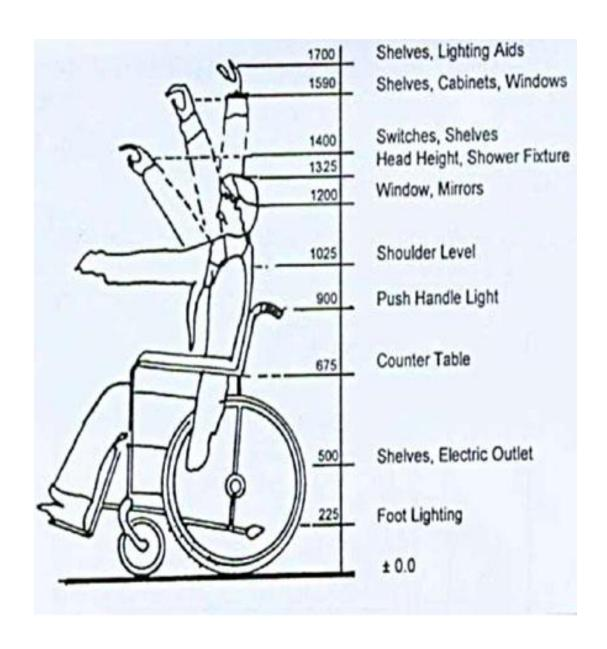
Fig-2. Typical Dimensions for Essential Uses with in easy reach
